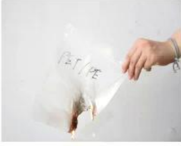
Showing the product polyoefin incineration
