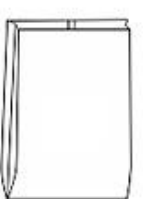
Fin/lap seal with side gusseted pouch
